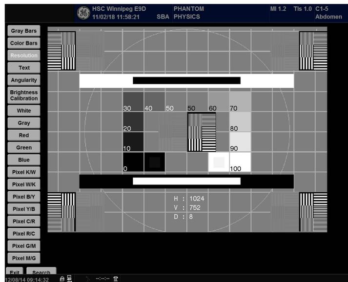
**Figure** SMPTE pattern on the GE Logic E9.
